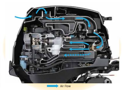
To help reduce the temperature inside of the engine cover, the rotating flywheel pushes warm air inside of the cover through the vent hole to the outside.
