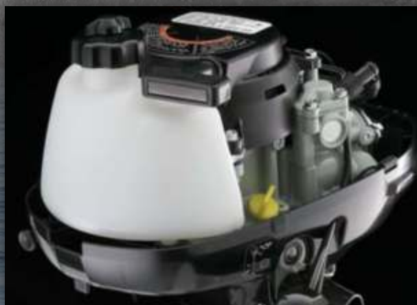
2.5HP single Cylinder OHV 4-stroke with 68cm3
